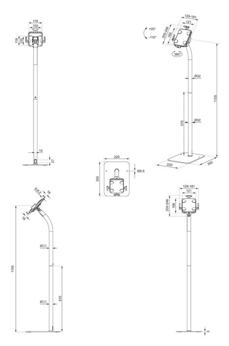
Neomounts Measuring unit: mm
