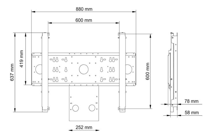
Neomounts Measuring unit: mm
