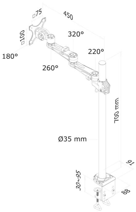
Neomounts Measuring unit: mm
