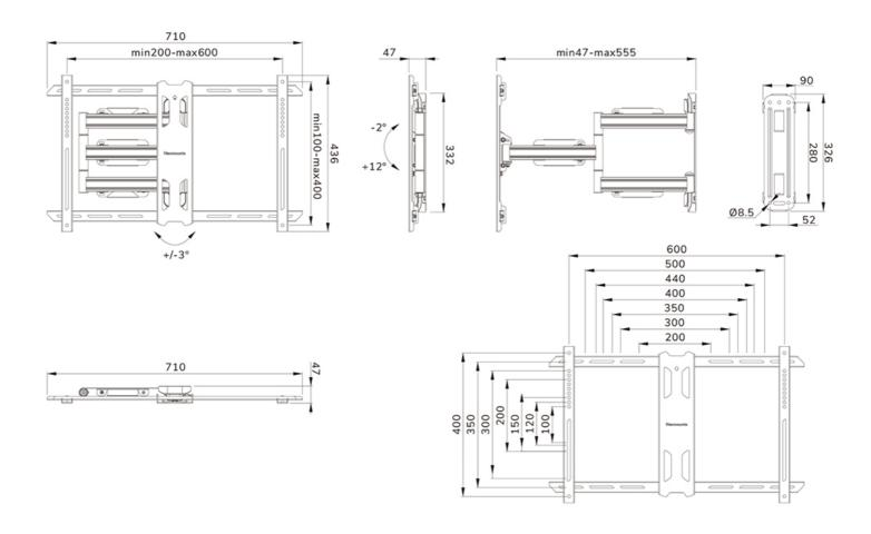
Neomounts Measuring unit: mm
