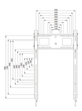
Neomounts Measuring unit: mm
