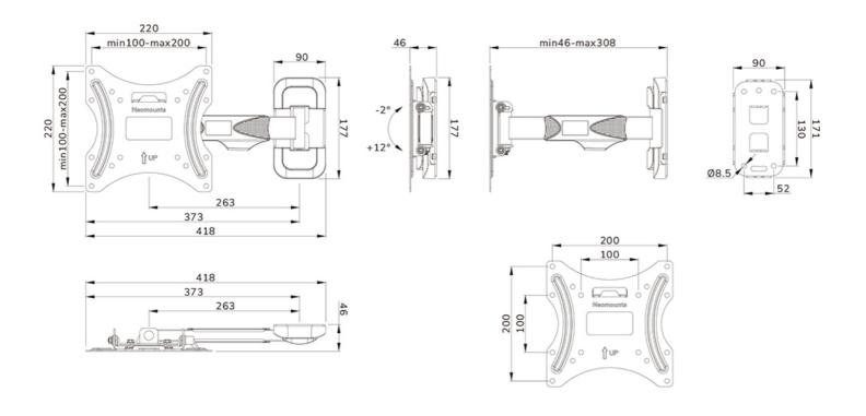
Neomounts Measuring unit: mm
