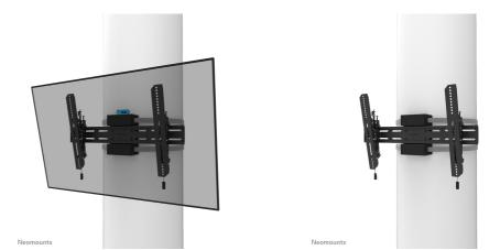
Neomounts WL35S-910BL16 Tiltable TV pillar mount - 40-75" - max 50 kg - VESA 300x100-600x400 - suitable for Ø 25-100 cm - d 6,9 cm - level adjustment - lockable (incl. security screw, excl. lock) - black
